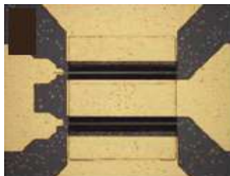
Fig. 22: The optical microscopic image of NCA HEMT structure. [33]
