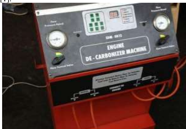
Fig. 5: Chemical Decarbonisation system
