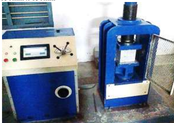
Fig. 9: Compression Testing Machine
