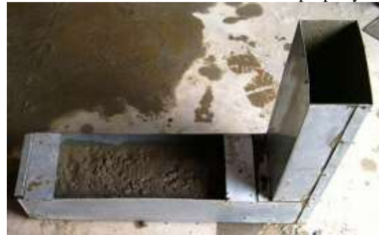
Fig. 8: Flow through rebar in L-Box
