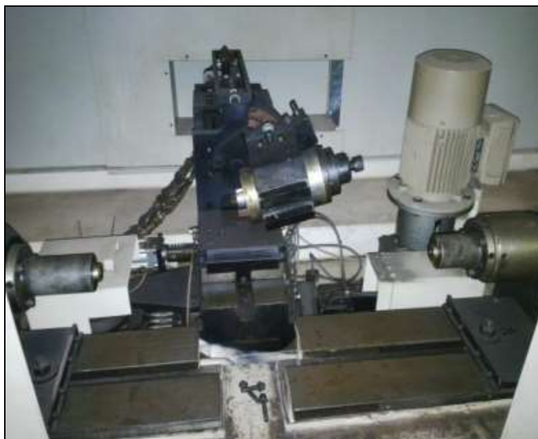
Fig. 3: Gear Burnishing Set up
