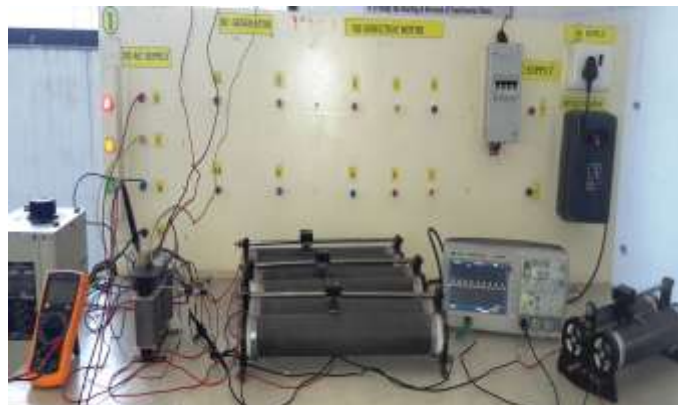
Fig. 1: Hardware Implementation of Transformer with injection of DC Current
