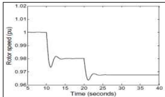
Fig. 10: Rotor speed variation with load
