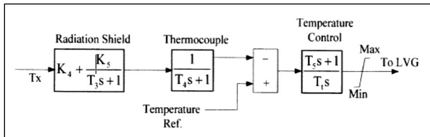
Fig. 2: temperature control of microturbine
