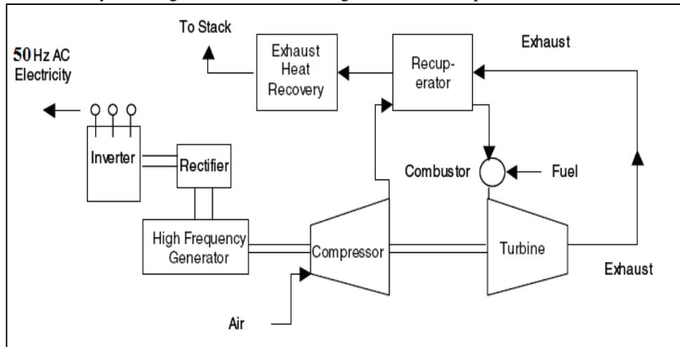
Fig. 1: Basic component of Microturbine
