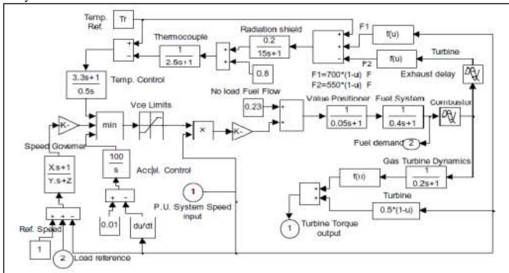
Fig. 4: Simulink implementation of microturbine
