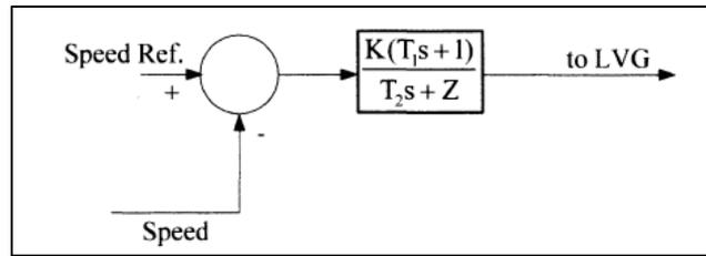
Fig. 3: speed control of microturbine
