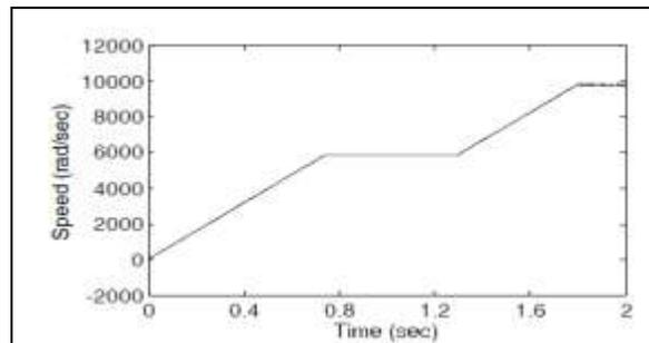
Fig. 8: motoring and generating operation speed variation of PMSG
