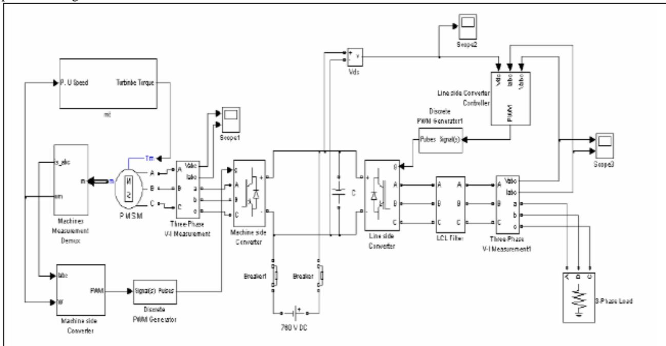
Fig. 5: microturbine generator system implementation in SimPower system
