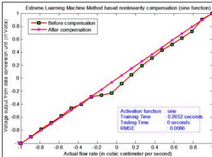
Fig. 5: ELM based nonlinearity compensation (sine)
