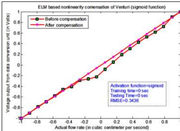
Fig. 6: ELM based nonlinearity compensation (sigmoid)
