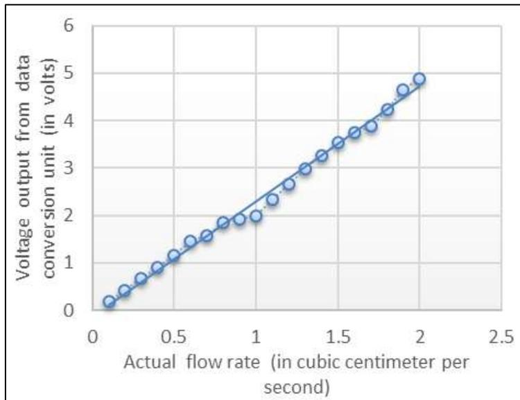
Fig. 3: Input-Output characteristics of flow transducer
