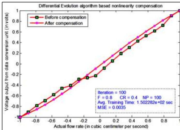
Fig. 8: DE based nonlinearity compensation
