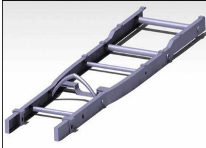
Fig. 15: Modified C section chassis
