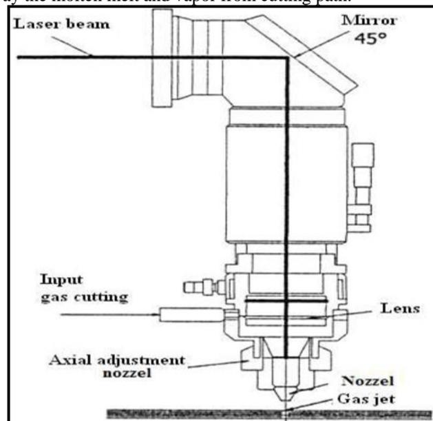
Fig. 1: Laser Beam Cutting
