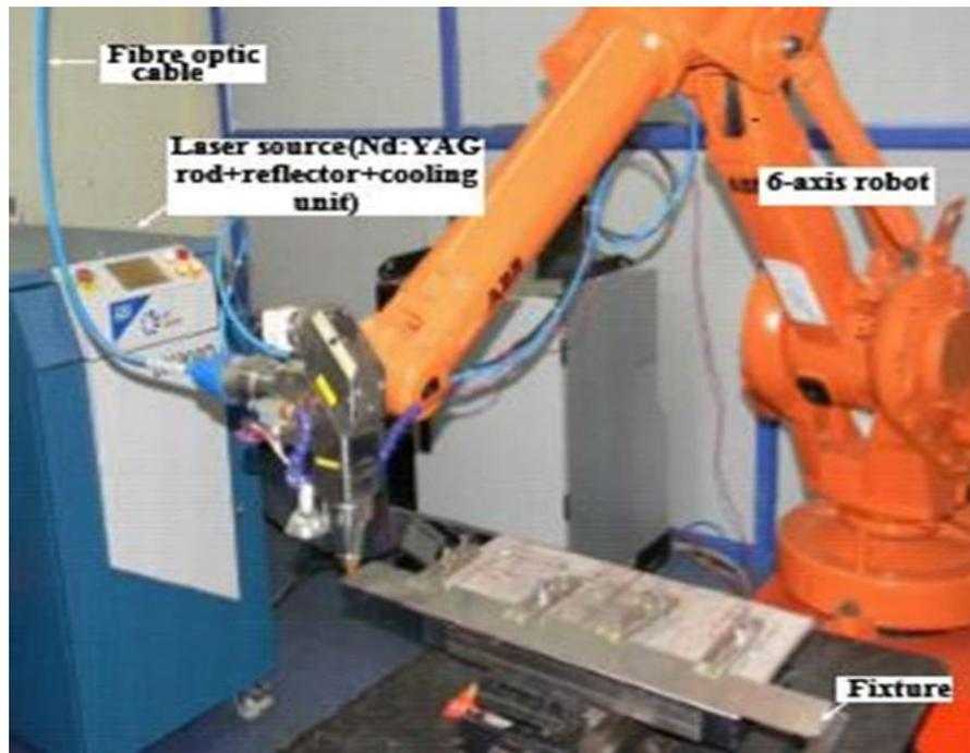
Fig. 2: Laser Cutting Setup
