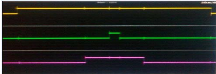
Fig. 9: Symmetric waveform of SVPWM
