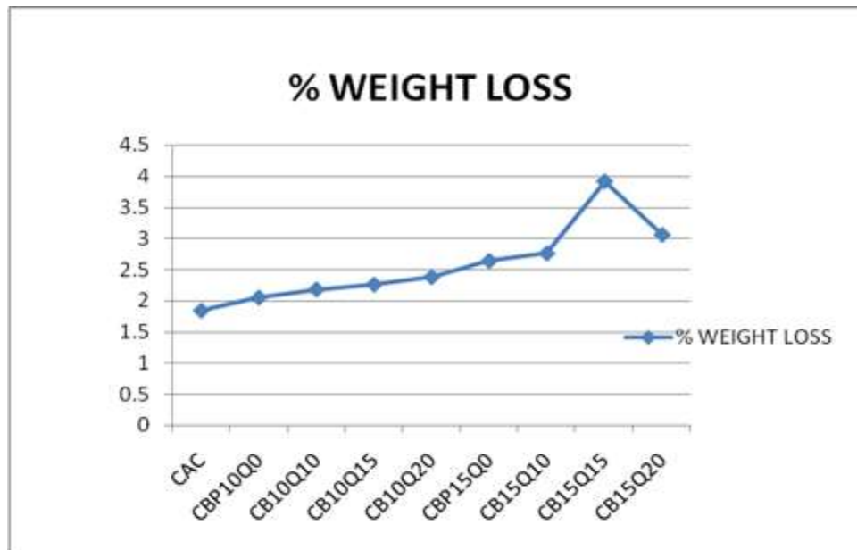
Fig. 7: Effect of Sulphuric acid (28 days)
