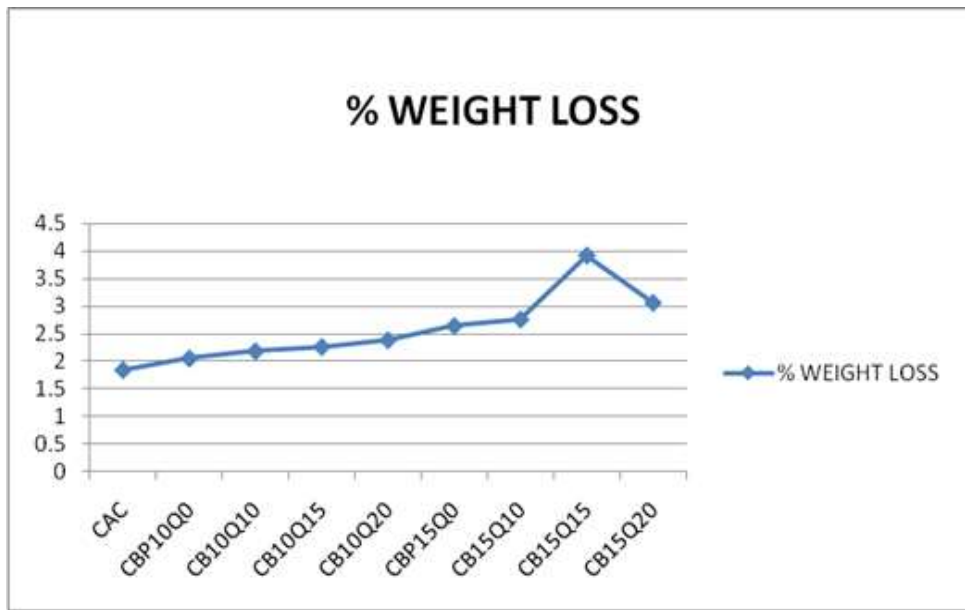
Fig. 6: Effect of Sulphuric acid (7 days)
