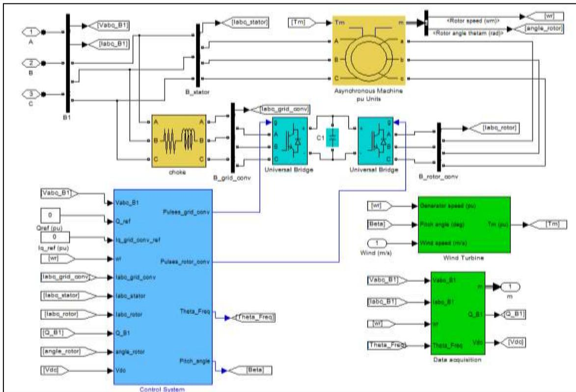
Fig. 3: Doubly fed induction generator wind turbine
