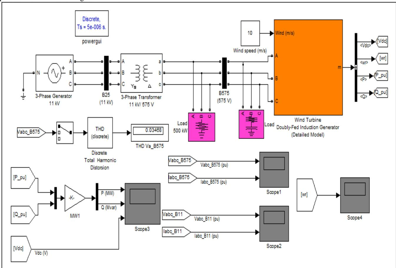
Fig. 2: Simulink model of fuzzy logic controller based WECS
