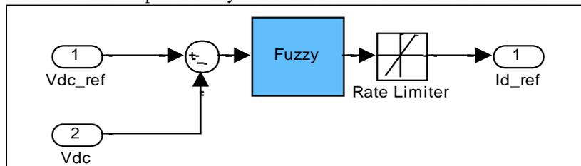
Fig. 6: Fuzzy based DC bus voltage regulator
