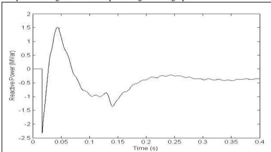
Fig. 12: Reactive power Vs time characteristics of fuzzy system
