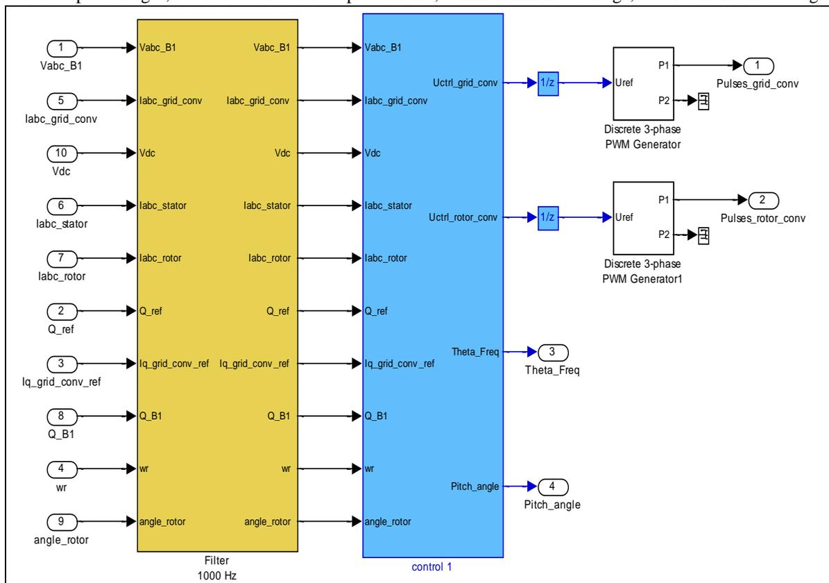
Fig.4. Back to back converter control system
