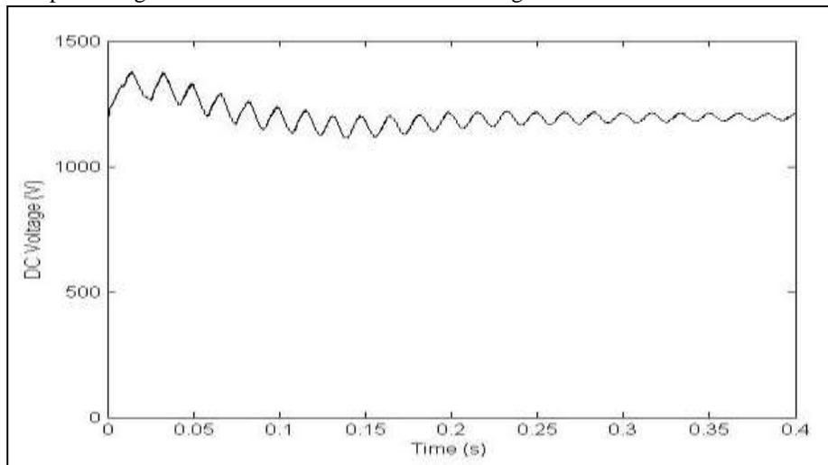
Fig. 13: Common link DC output voltage Vs time
