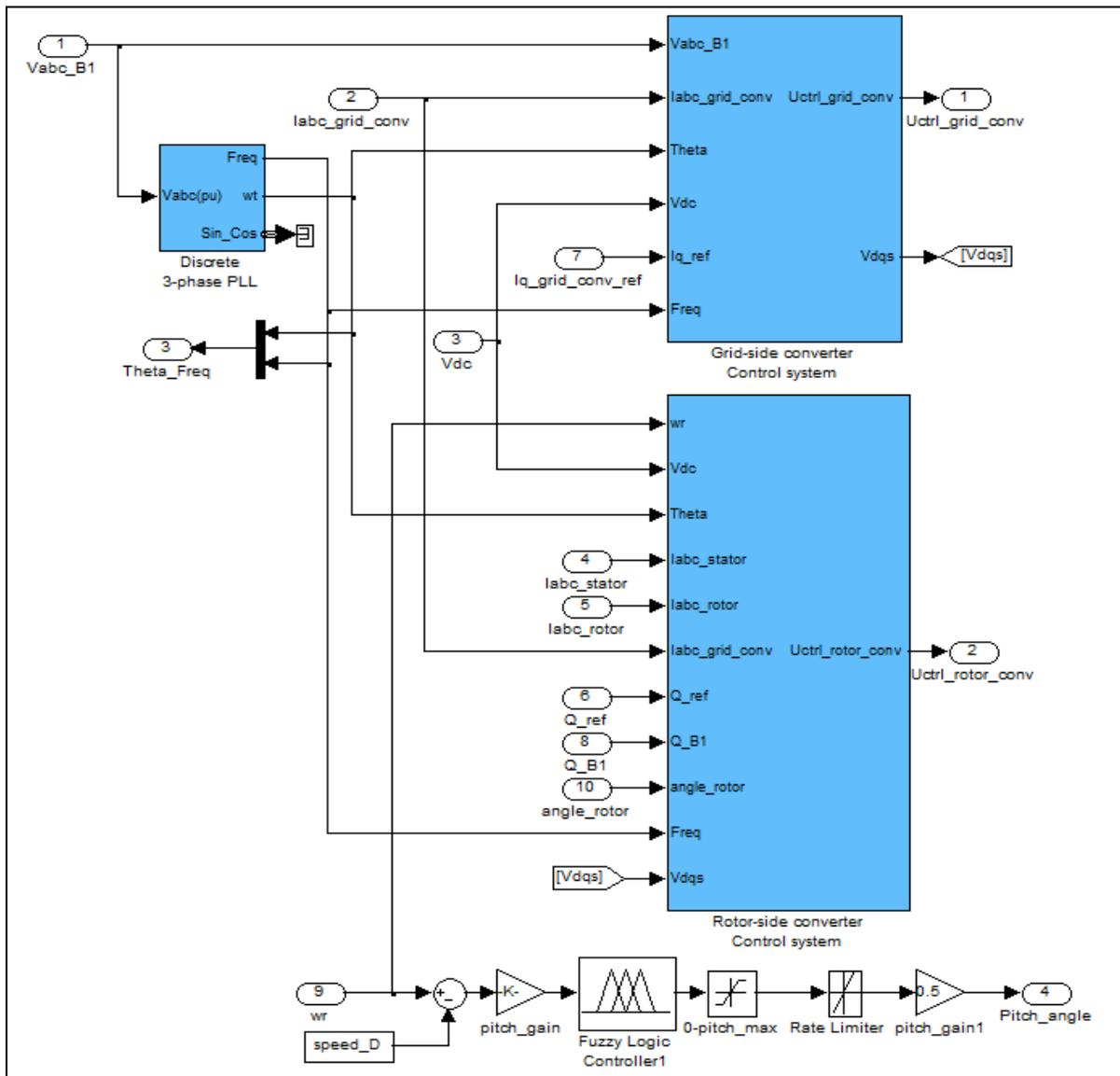
Fig. 5: Grid and rotor side control block
