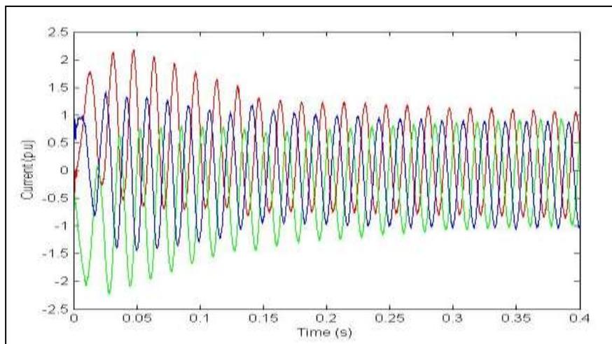
Fig. 8: Grid output current Vs time characteristics of fuzzy system
