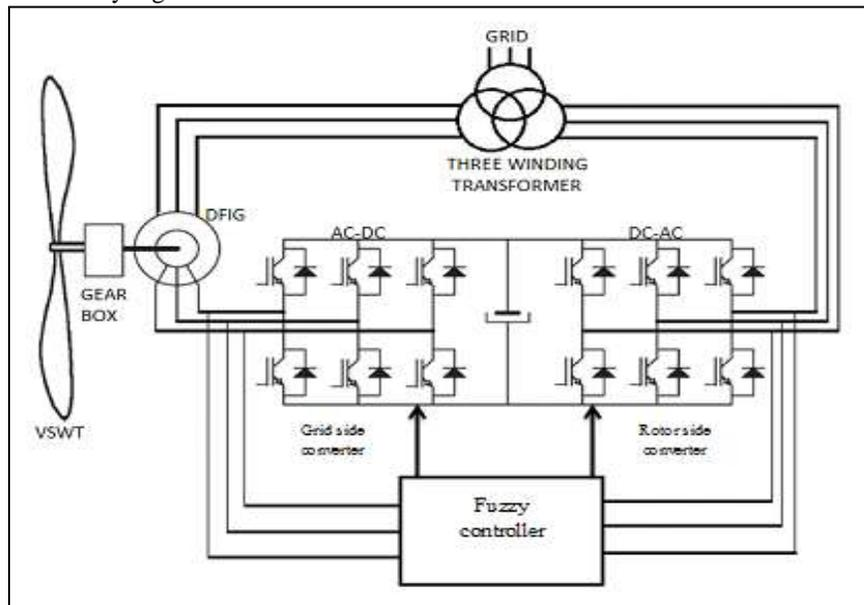
Fig. 1: Block diagram of fuzzy controller based WECS
