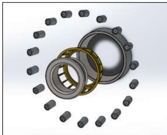
Fig. 3: Roller bearing made into model using Solidworks
