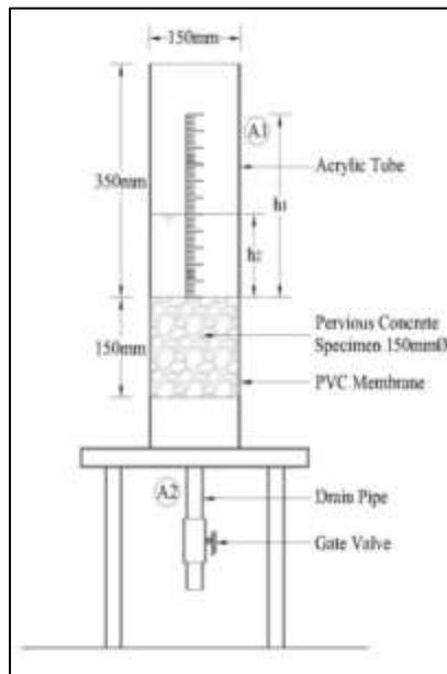
Fig. 3: Falling head permeability test setup
