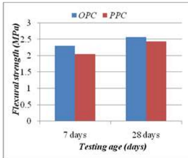
Fig. 6: Flexural strength
