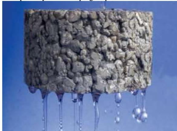
Fig. 1: Pervious Concrete
