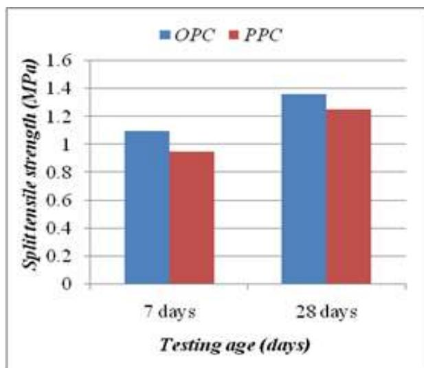
Fig. 5: Split tensile strength
