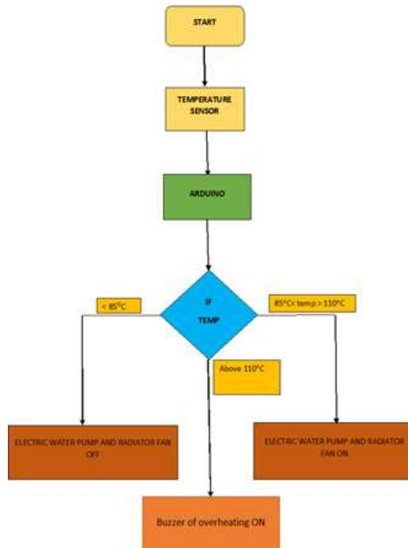
Fig. 8: Algorithm of the electronic circuit
