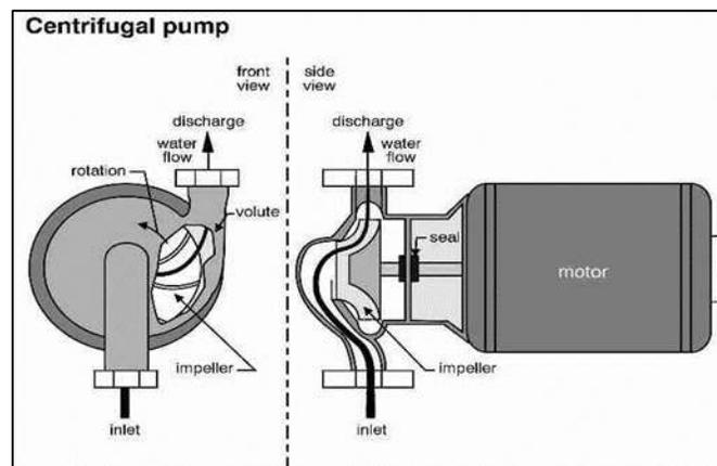
Fig. 3: Centrifugal type electric water pump
