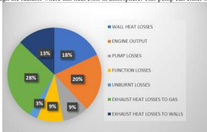
Fig. 1: Pie diagram of Overall losses in engine
