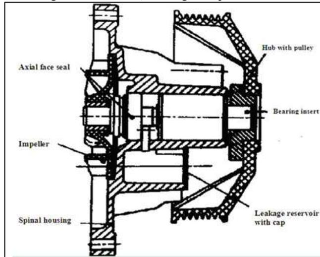
Fig. 2: Mechanical Water Pump
