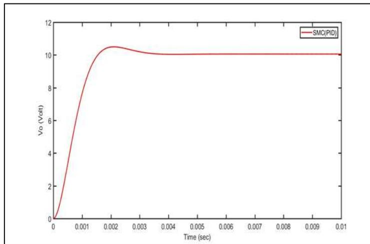
Fig. 4: Output voltage of Buck Converter with SMC using PID surface
