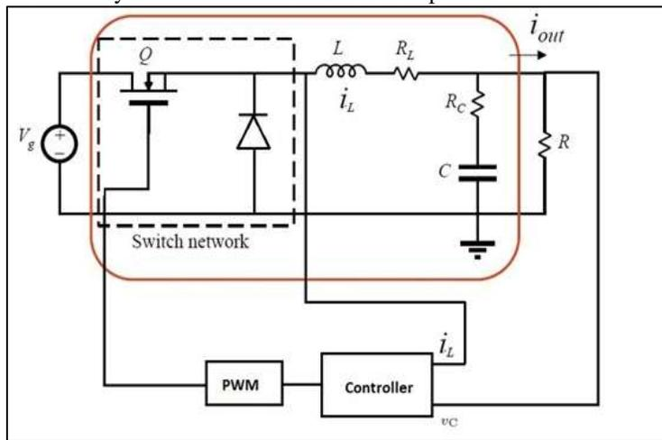
Fig. 3: Schematic Block Diagram of Simulation Model
