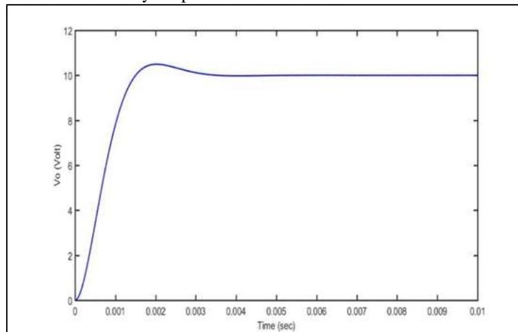
Fig. 6: Output voltage of Buck Converter using SMC with a disturbance in input voltage.
