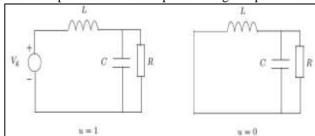
Fig. 2: DC-DC Buck Converter during ON and OFF state
