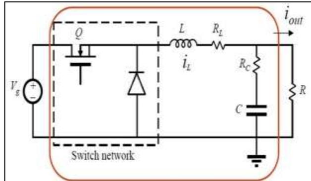
Fig. 1: Buck Converter System
