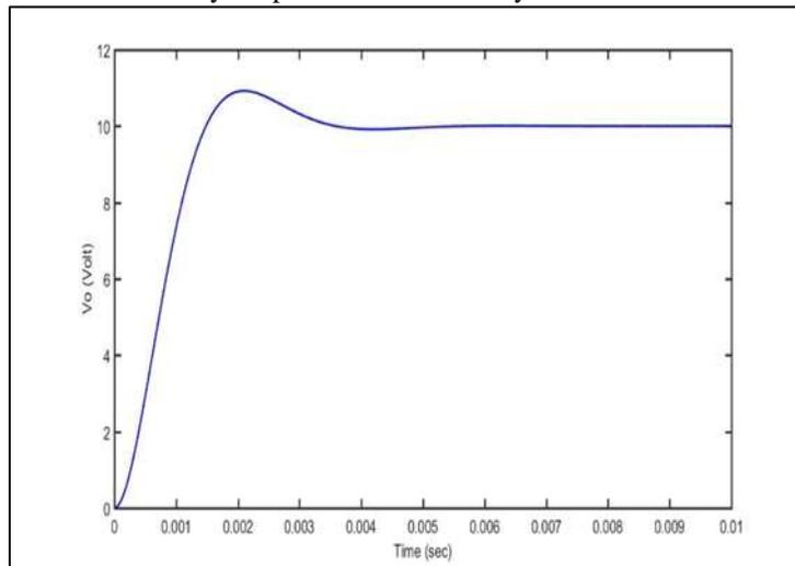
Fig. 8: Output voltage of Buck Converter using SMC with a disturbance in capacitor
