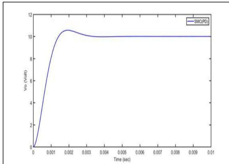
Fig. 5: Output voltage of Buck Converter with SMC using PD surface
