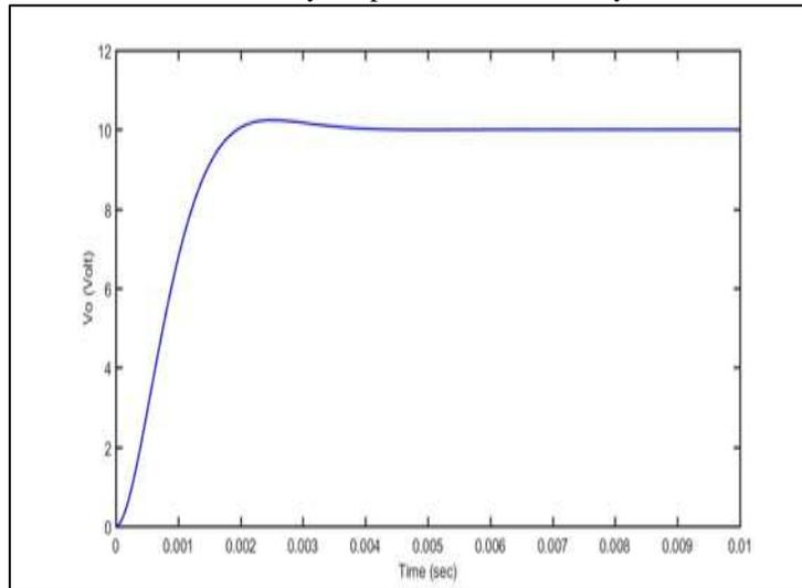
Fig. 7: Output voltage of Buck Converter using SMC with a disturbance in inductor.
