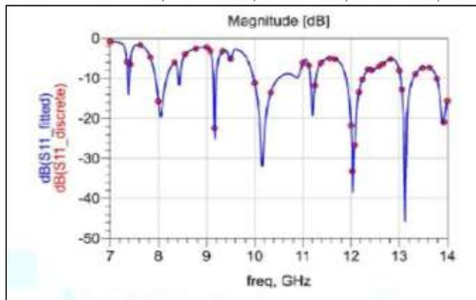
Fig. 3: S parameter of circular patch antenna
