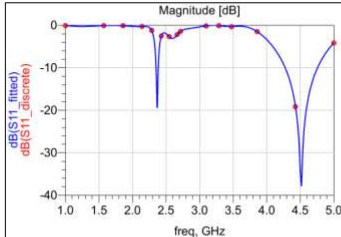
Fig. 4: S parameter of triangular patch antenna
