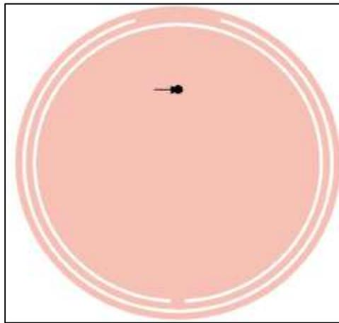
Fig. 1: circular patch antenna
