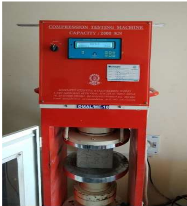
Fig. 1: Test setup for testing of cubical specimen
