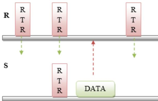
Fig. 4: RTR and DATA Packets between a Receiver (R) and a Sender (S)
