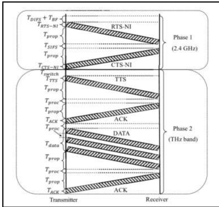
Fig. 5: Assisted beamforming MAC for Terahertz networks [15]
