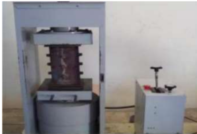
Fig. 4b: Experimental setup for push out test
