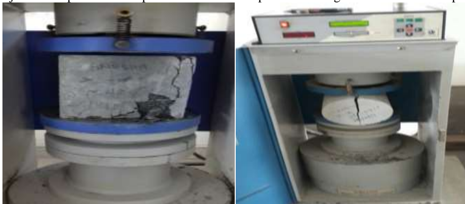
Fig. 1: Image of Cube and Cylinder specimen tested in Compressive Testing Machine (CTM).
