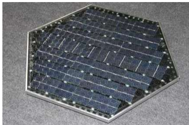
Fig. 2: One hexagonal solar panel showing the inner PV cells and LEDs.
