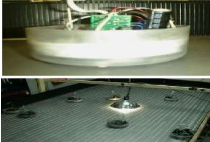
Fig. 3: Our 4” diameter robot picks up power from its environment and learns while on-line.
