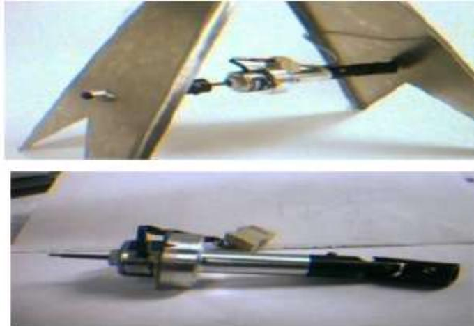
Fig. 1: Prototype “living truss” robot and detail of linear motor assembly
