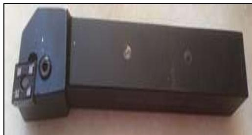
Fig. 4: Tool Holder PCLNR 2020 M12
