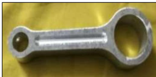
Fig. 4: Finished component of connecting rod after machining
