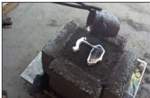
Fig. 3: pouring of molten composition in to die
