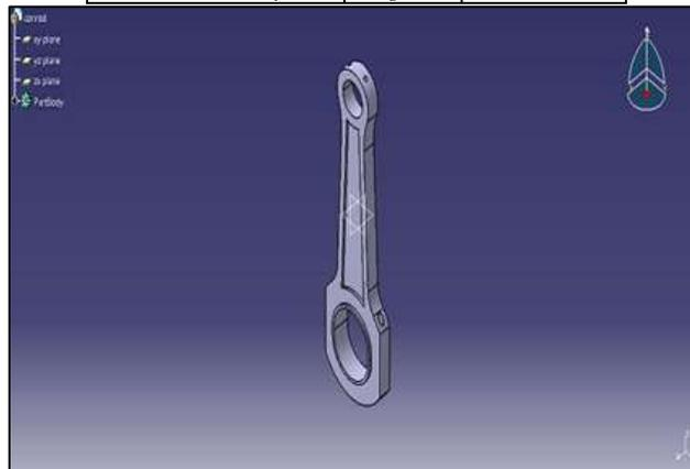
Fig. 1: modeling of connecting rod using Catia -software
