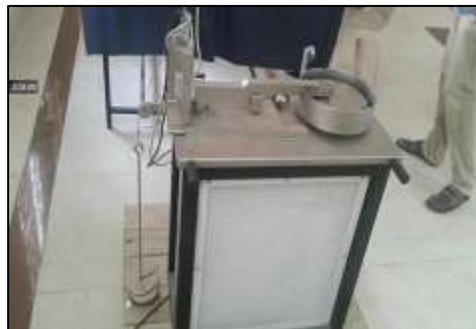
Fig. 6: experimental set up of Pin-on-disc wear tester (Model: Ducom TR- 20 LE)
