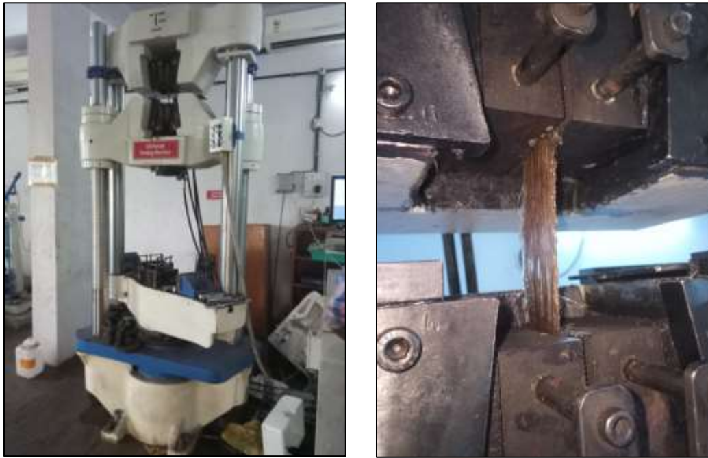
Fig. 4: Test conducted on machine & clamping of specimen
