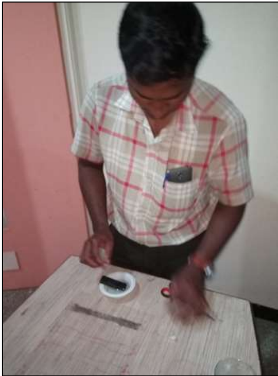
Fig. 2: Mixing of epoxy and hardener & Applying solution to specimen
