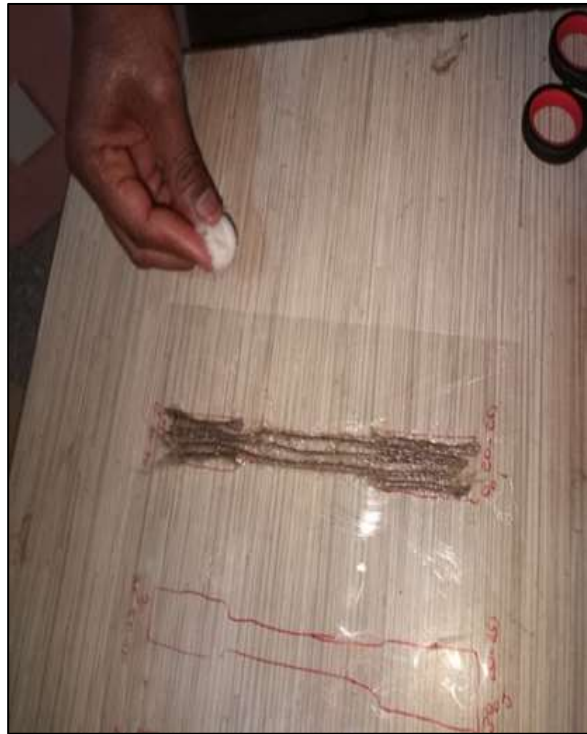
Fig. 2: Mixing of epoxy and hardener & Applying solution to specimen
