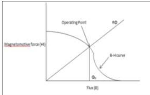
Fig. 5: Magneto motive force vs flux
