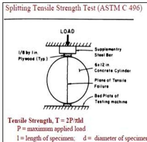
Fig. 6: Splitting Tensile Strength Test
