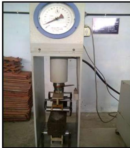
Fig. 5: Flexural Testing on Beam
