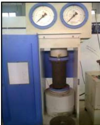
Fig. 4: Compression Testing on Cylinders
