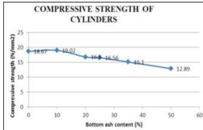
Fig. 8: Compressive Test of Cylinders
