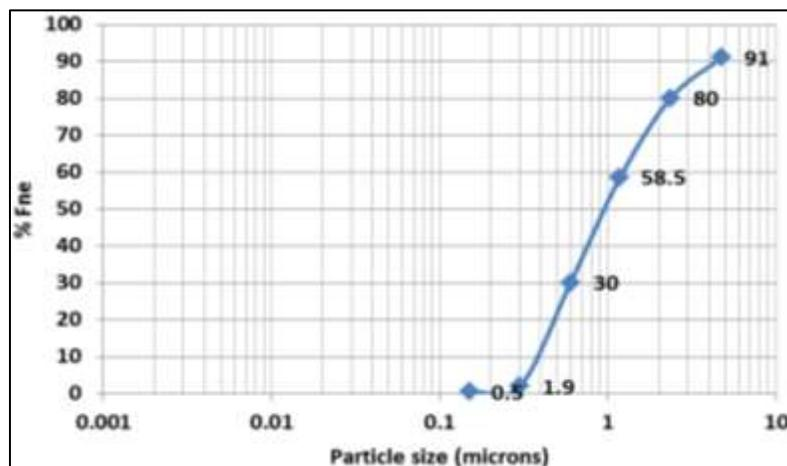
Fig. 2: Bottom Ash particle size distribution curve
