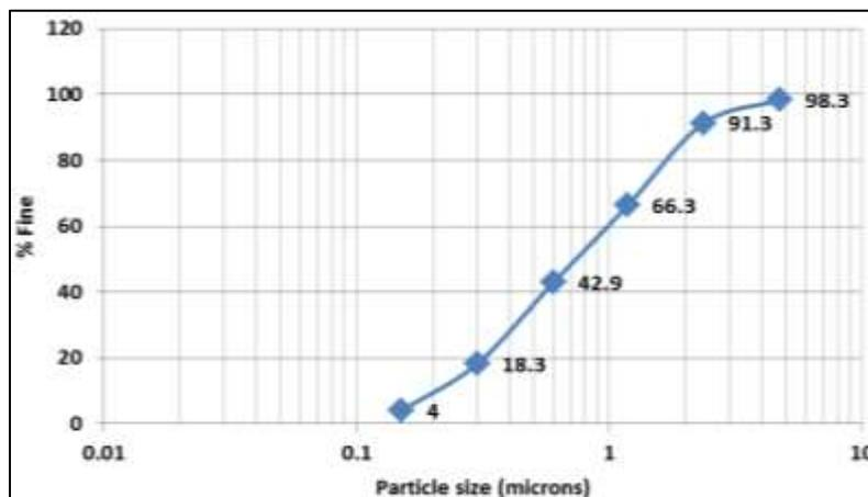
Fig. 1: Fine aggregate particle size distribution curve
