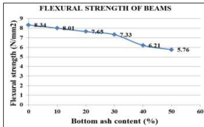
Fig. 9: Flexural Strength on Beams
