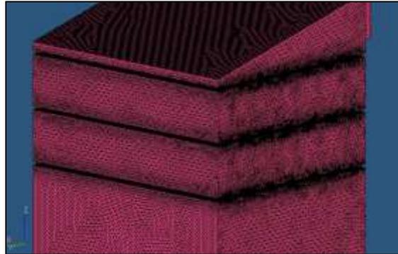
Fig. 6.2: Meshing of Solar cabinet dryer
