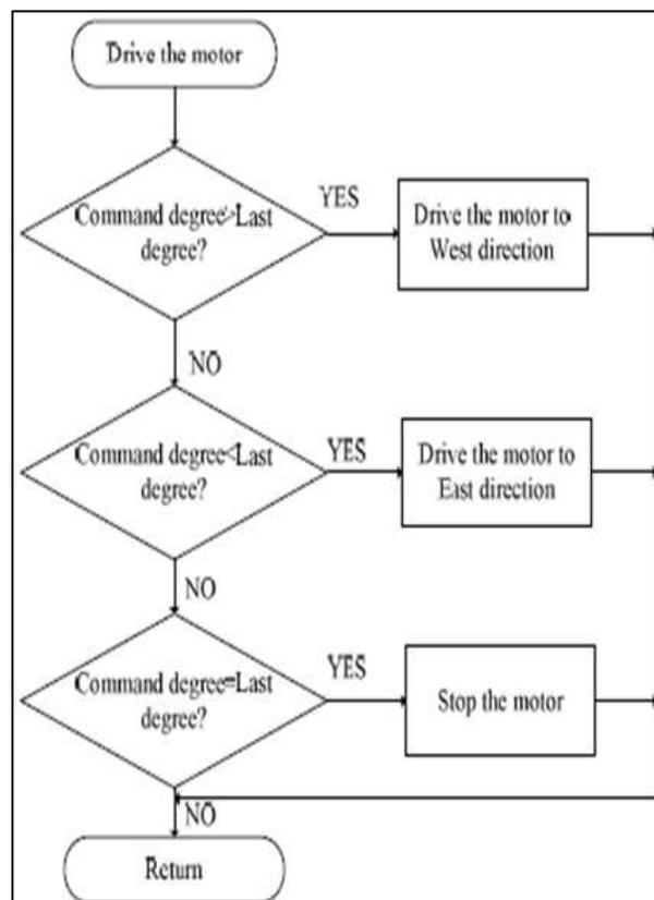
Fig. 6: Flow Chart for the Motor Operation
