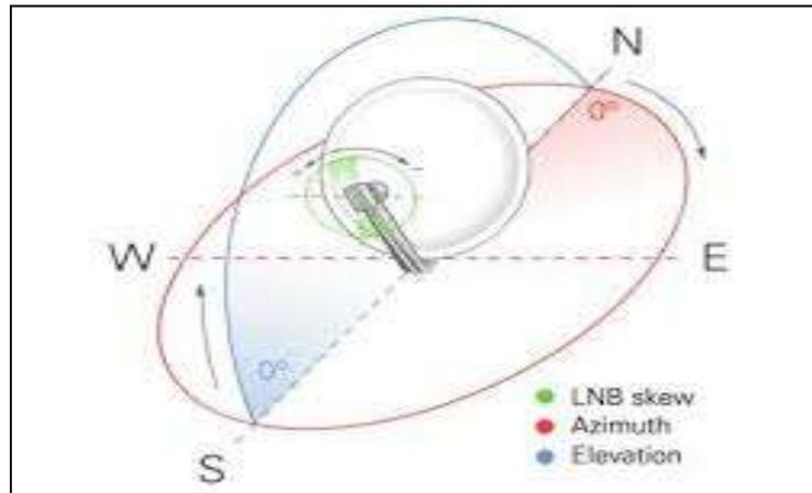
Fig. 4: Aligning the Dish
