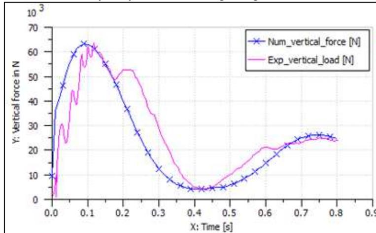
Fig. 6: Vertical Force Vs Time Curves of MLG Comparison
