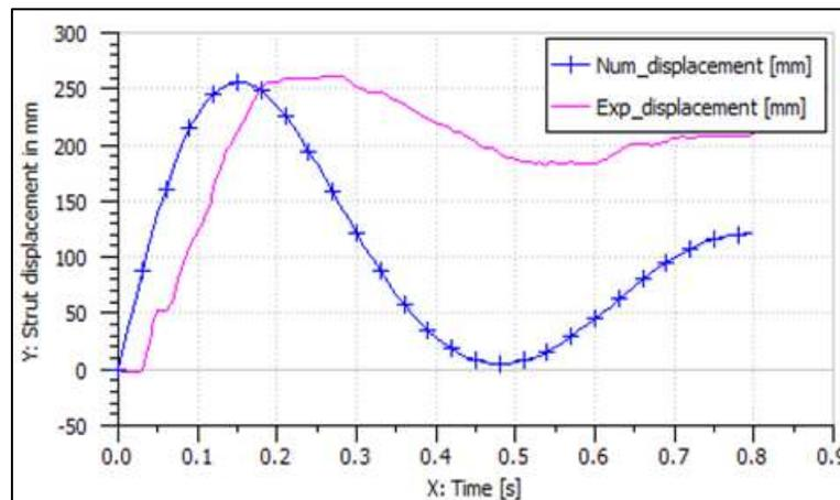
Fig. 7: Strut Displacement Vs Time Curve of MLG Comparison
