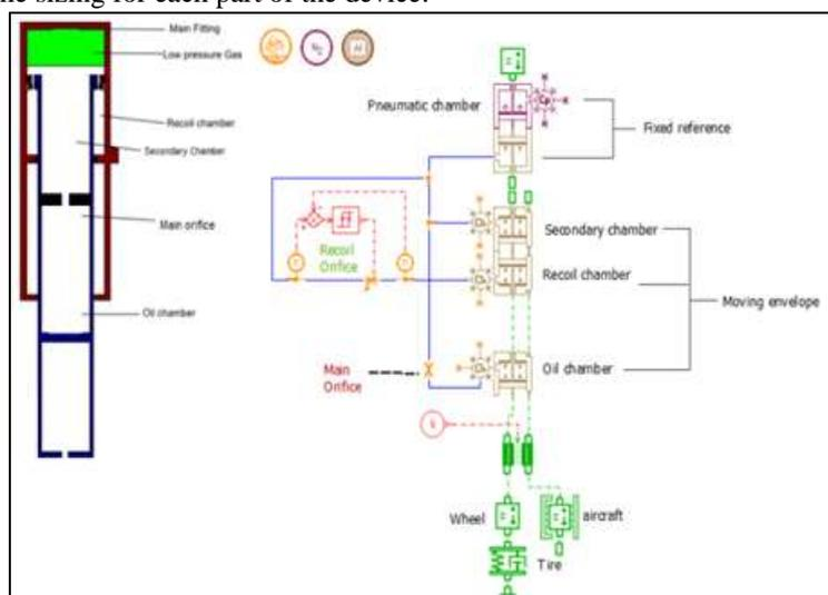
Fig. 4: Principle Scheme & AMESim Model
