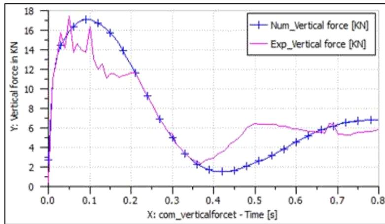
Fig. 8: Vertical Force Vs Time Curve of NLG Comparison
