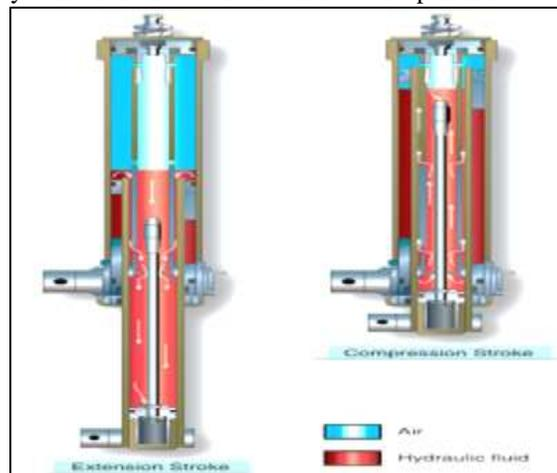
Fig. 2: Cut section View of Shock Strut
