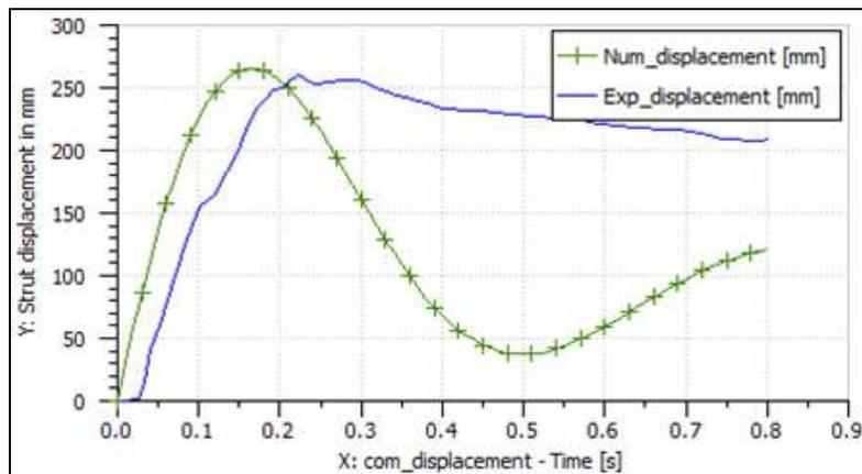
Fig. 9: Strut Displacement Vs Time Curve of NLG Comparison
