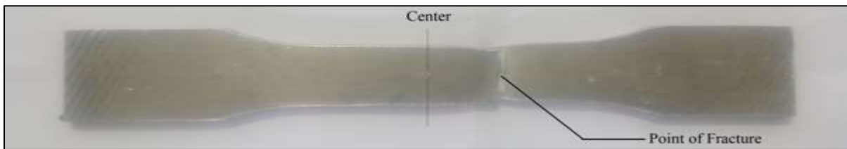
Fig. 1: Tensile specimen of base metal after fracture
