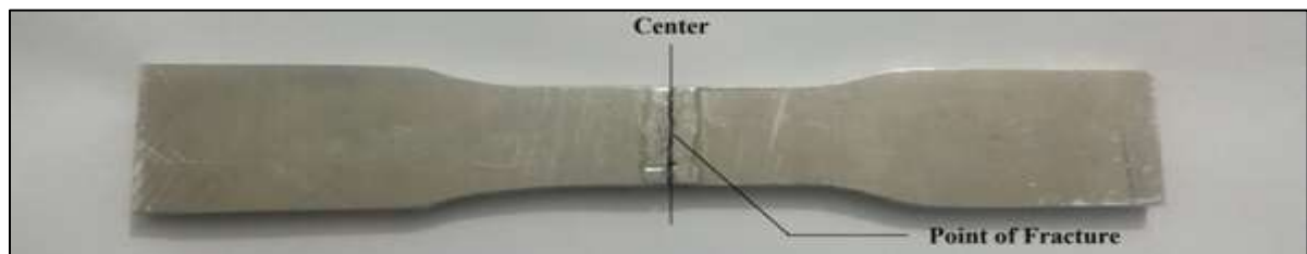
Fig. 2: Tensile specimens of TIG welded joint after fracture
