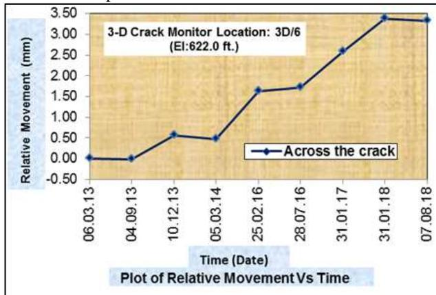
Fig. 5: Graphical pattern of 3D Crack Monitor
