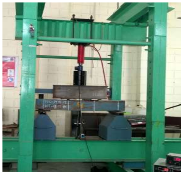
Fig. 13: Testing of Composite beam with stud-shear connectors.
