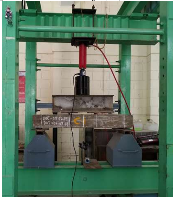
Fig. 12: Testing of Conventional beam.
