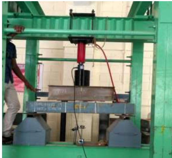
Fig. 14: Testing of Composite beam with Channel-shear connectors.
