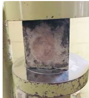
Fig. 9: Failure on cube.
