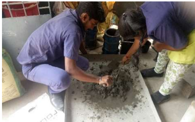
Fig. 6: Mixing of concrete for cube and cylinder casting
