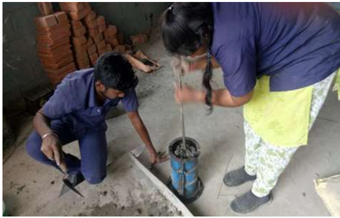
Fig. 7: Casting of Cylinder
