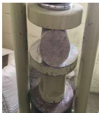
Fig. 10: Split tensile loading on cylinder.
