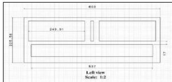
Fig. 3.6: Modified frame design: side view
