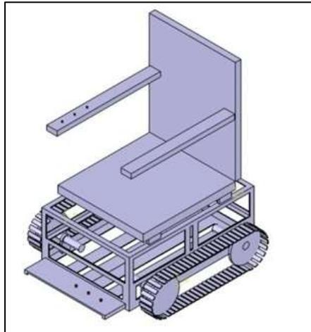
Fig. 3.14: CAD model of the wheelchair
