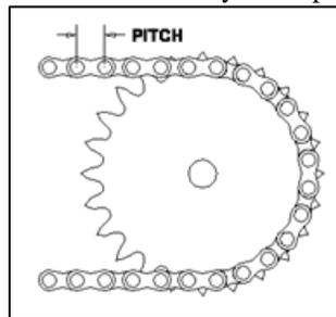
Fig. 3.10: Chain movement over the sprocket
