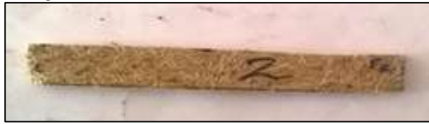
Fig. 9: Impact Test Specimen before Testing
