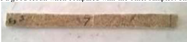
Fig. 5: Water Absorption Test Specimen Before Testing
