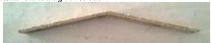
Fig. 6: Water Absorption Test Specimen After Testing
