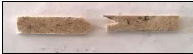
Fig. 10: Impact Test Specimen after Testing
