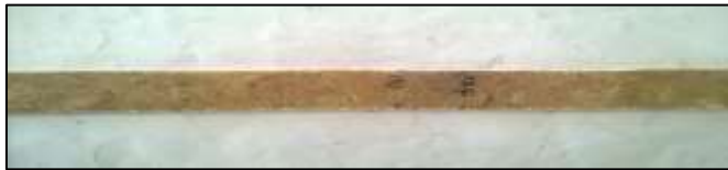
Fig. 1: Tensile Test Specimen before Testing
