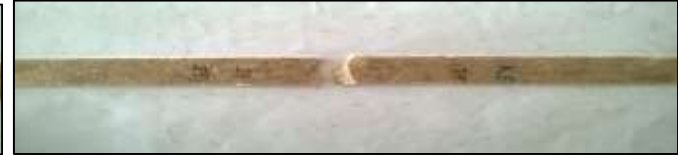
Fig. 2: Tensile Test Specimen after Testing
