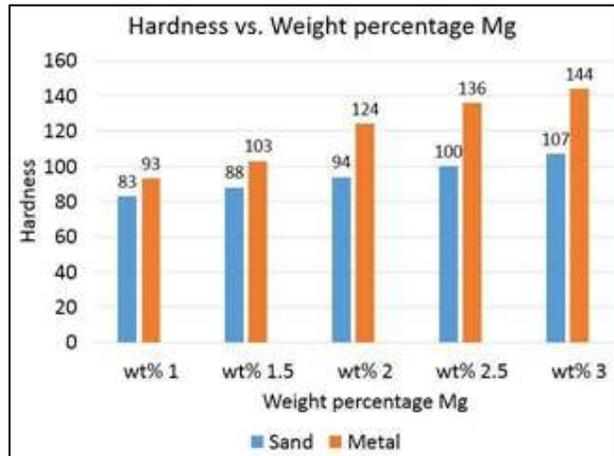
Fig. 3.6: Hardness vs. Weight Percentage
