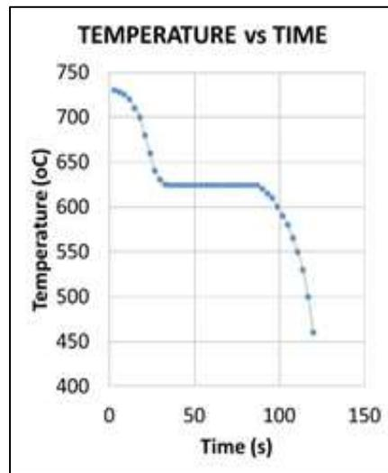
Fig. 3.10: Cooling Curve of Casting in Metal Die
