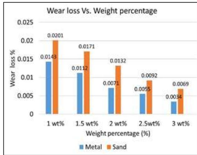
Fig. 3.9: Wear loss V.s Weight percentage
