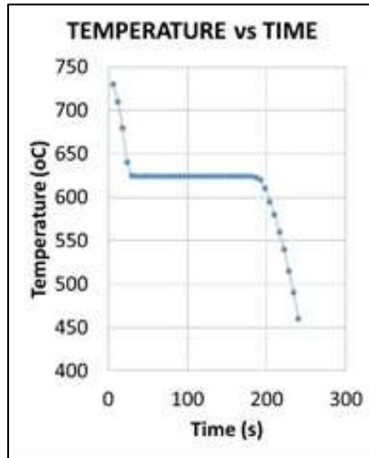
Fig. 3.11: Cooling Curve of Casting in Sand Die
