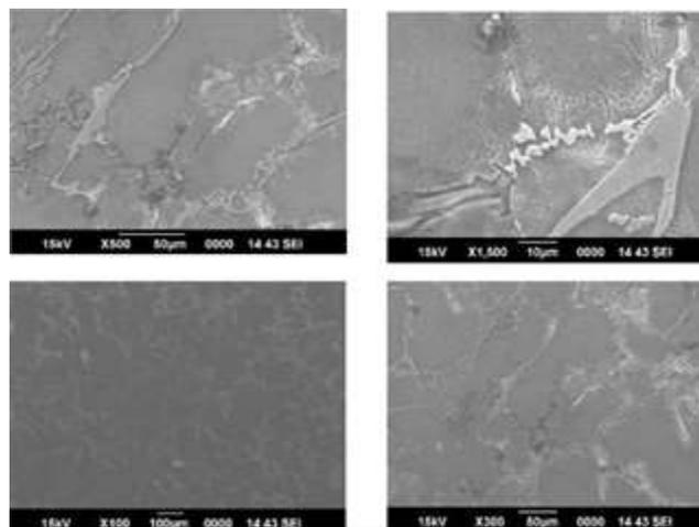
Fig. 3.13: SEM Image of 3 Wt % Sand Mould Casting
