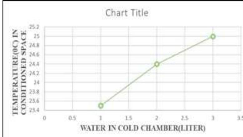
Fig. 13: Variation of temperature inside conditioned space
