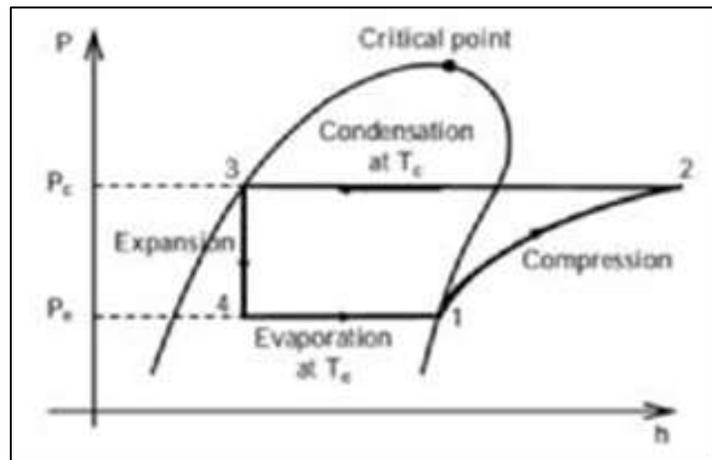
Fig. 1: Vapour compression cycle in p-h coordinates
