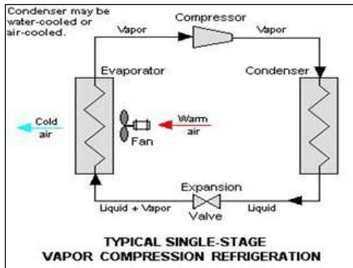
Fig. 2: Parts of typical vapour compression refrigeration
