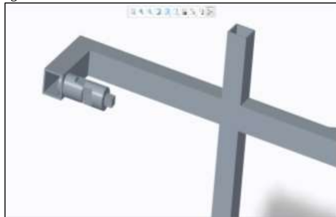
Fig. 3: Shoulder joint connected with universal joint
