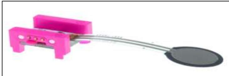
Fig. 5: Pressure Sensor
