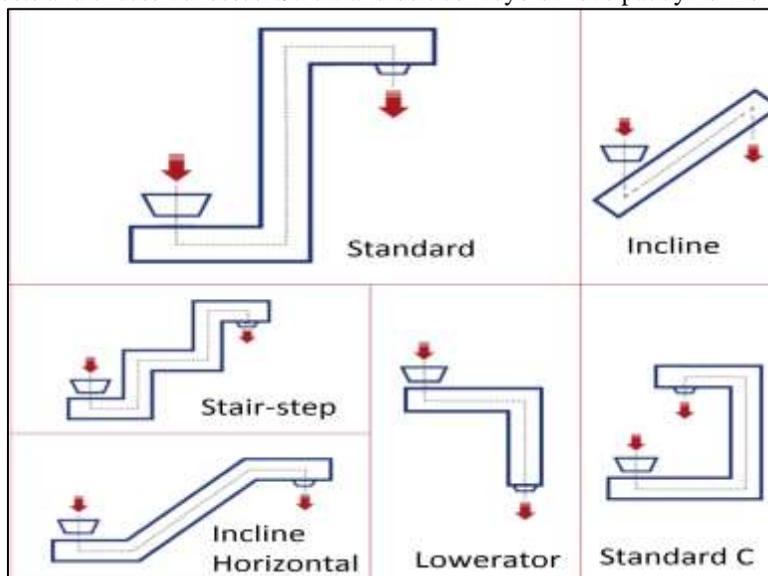
Fig. 1: Designs of Bucket Elevators
