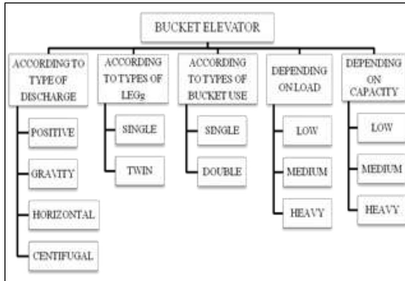
Fig. 2: Classifications of Bucket Elevators
