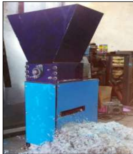
Fig. 6: Plastic Shredding Process
