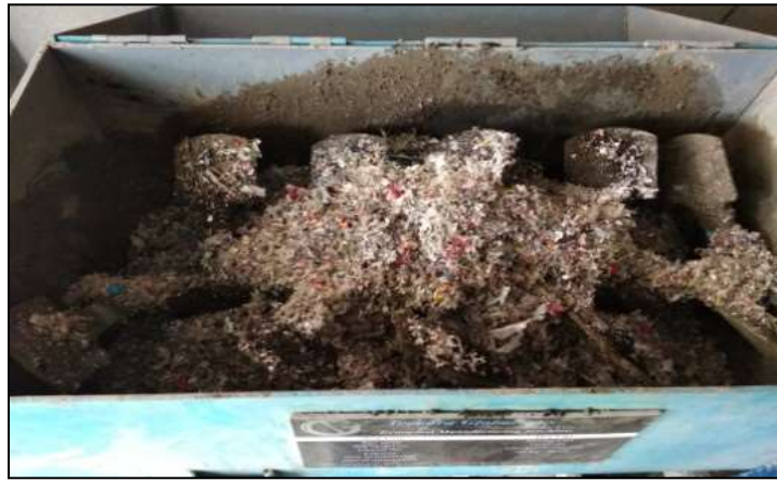
Fig. 7: Plastic Granules, Cement, Crush Sand & ECO in Mixing Unit
