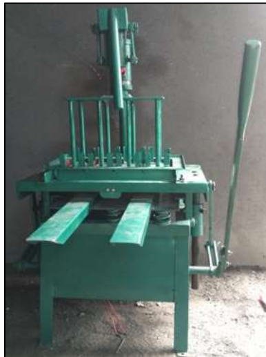
Fig. 3: Manual Brick Manufacturing Unit
