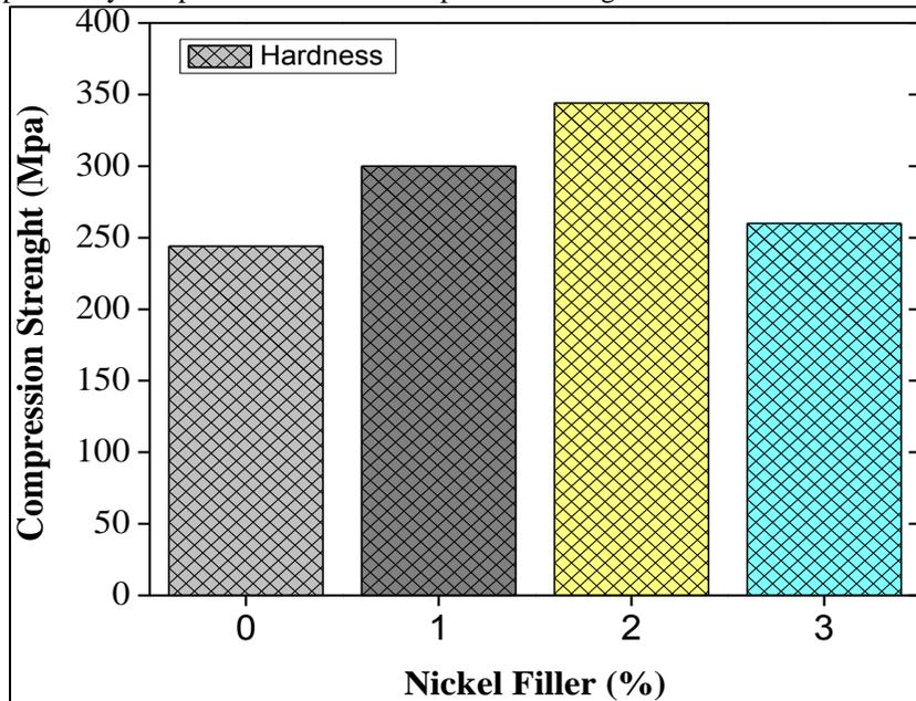
Fig. 1: Effect of Compressive Strength on Ni Metal Powder Filled Composites 5083 Aluminum Alloy Composites
