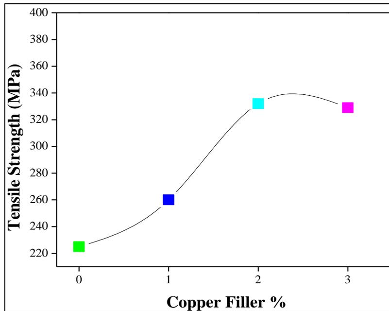
Fig. 6: Effect of Tensile Strength on Copper Metal Powder Filled 5083 Aluminum Alloy Composite
