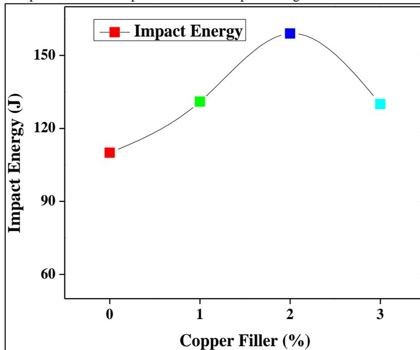
Fig. 5: Effect of Impact Strength on Copper Powder Filled 5083 Aluminum Alloy Composites
