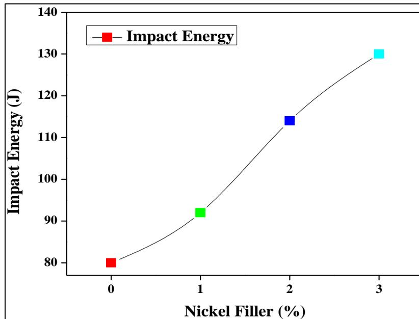
Fig. 2: Effect of Impact Strength on Nickel Powder Filled 5083 Aluminum Alloy Composites
