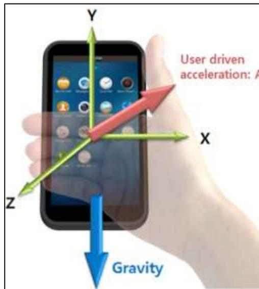
Fig. 2: Accelerometer Directions on a Smartphone
