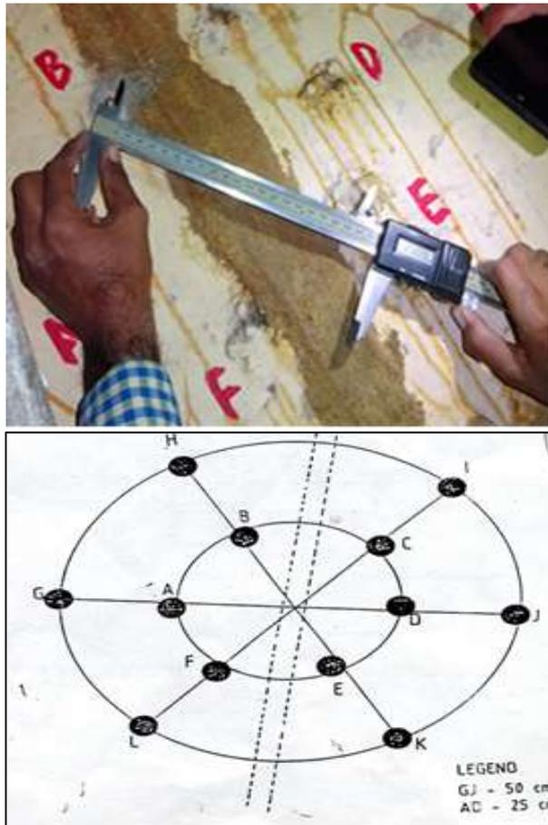
Fig. 2: 2-Dimensional crack monitor with axis orientation for monitoring of crack movement
