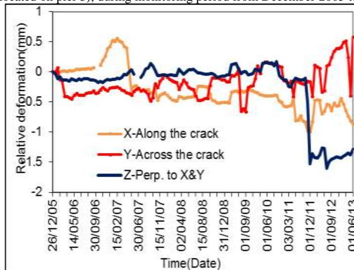
Fig.4: 3-D crack movement 3D/9, P3, S2
