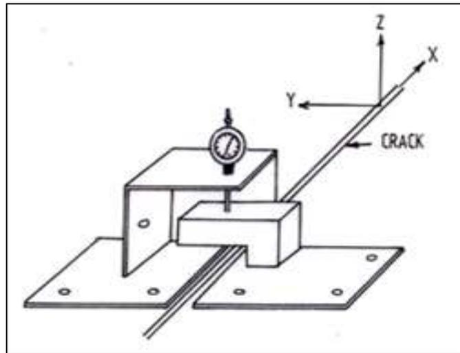
Fig. 3: 3-Dimensional crack monitor with axis orientation for monitoring of crack movement
