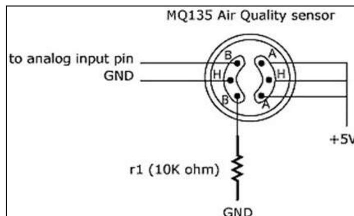
Fig. 1: MQ-135 Air Quality Sensor
