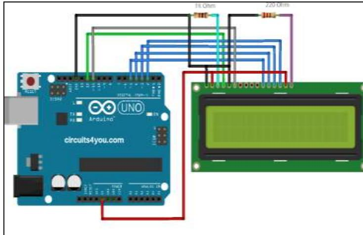
Fig. 4: Interfacing Arduino to Display
