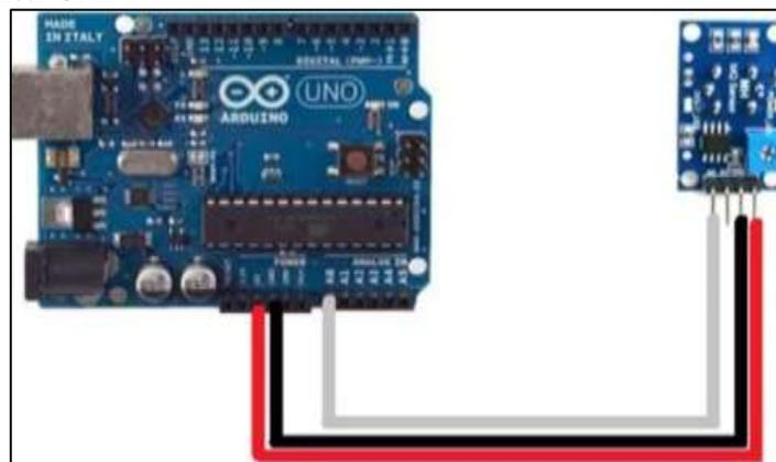
Fig. 5: Interfacing Arduino with MQ135
