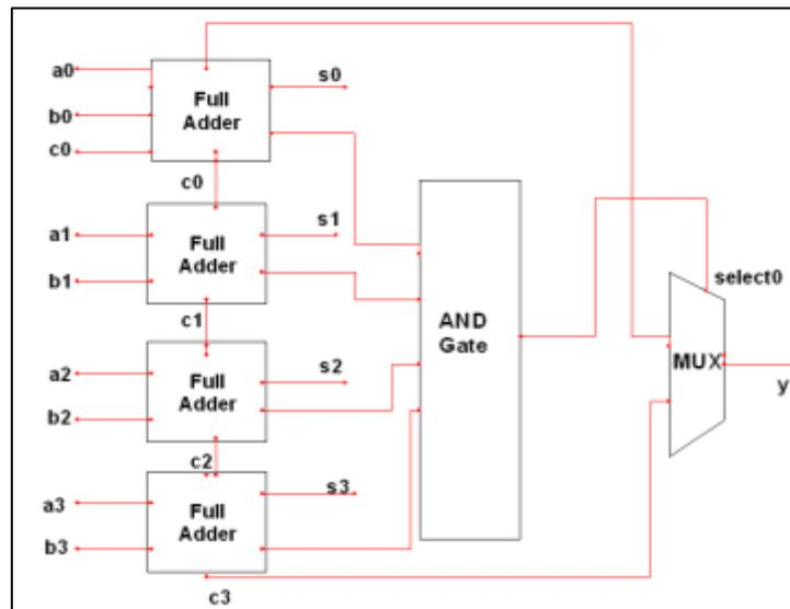
Fig. 2.1: Block diagram of Carry Skip Adder
