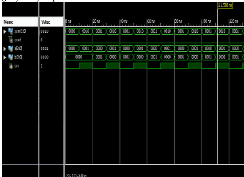
2) Waveform of CMOS design of Carry Skip Adder:
