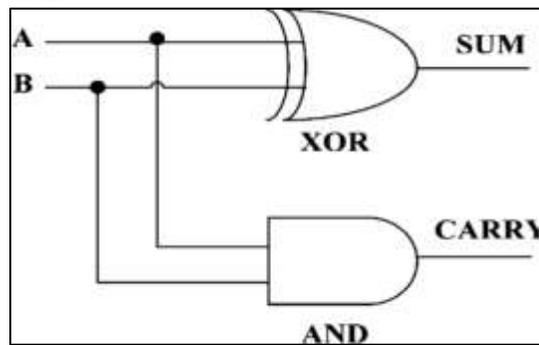
Fig. 1.2: Logic diagram of Half Adder:
