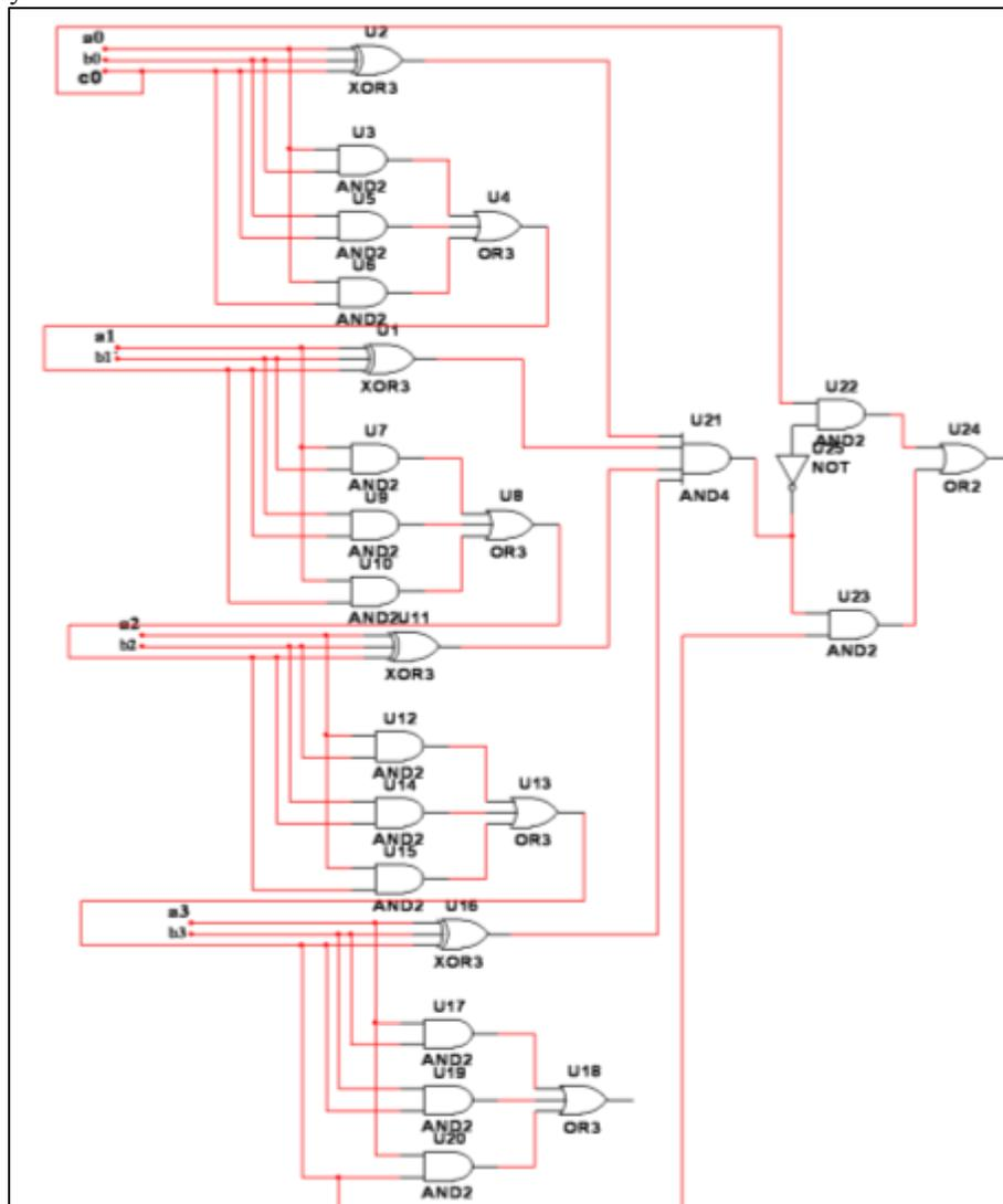
Fig. 2.2: Logic Diagram of Carry Skip Adder
