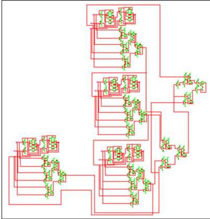
Fig. 2.3: CMOS Design o Carry Skip
