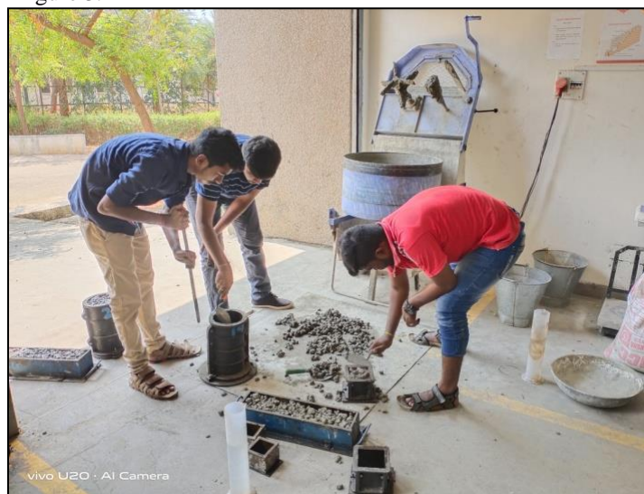
Fig. 3: Casting of Specimens
