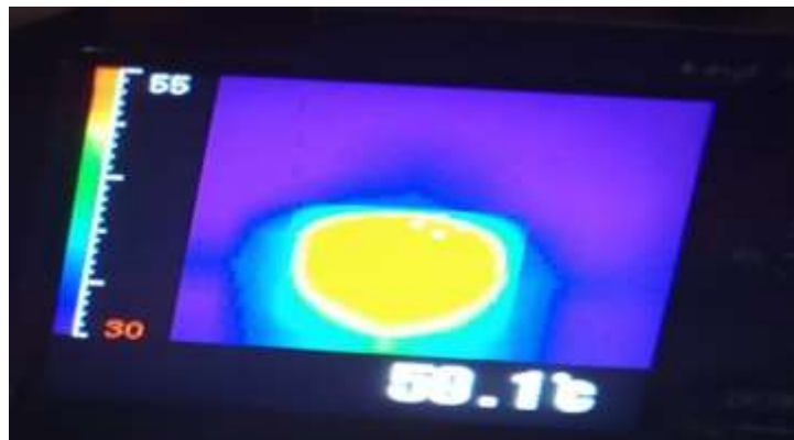
Fig. 4: Gas leak detection using thermal camera
