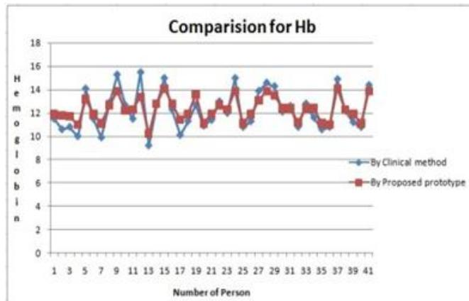
Fig. 4: Comparison for Manual and calculated Hb
