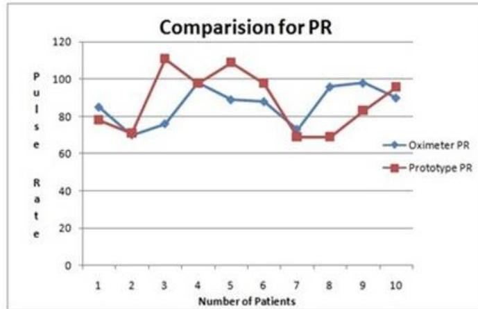
Fig. 2: Comparison for oximeter and prototype for PR
