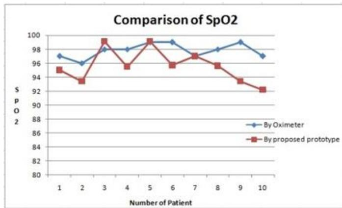
Fig. 3: Comparison for oximeter and prototype for SpO2
